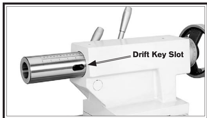
Figure 41. Drift key slot in the side of the quill.
